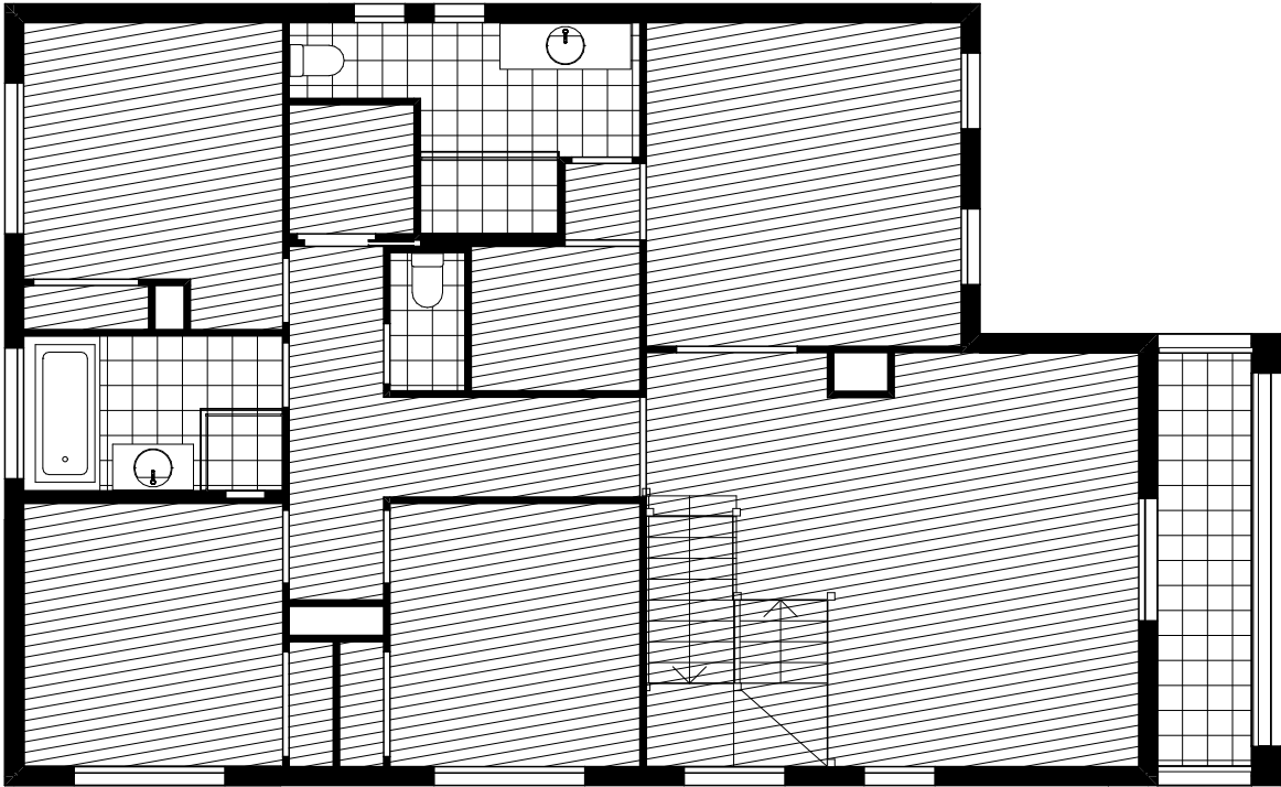
FLOOR COVERINGS (FIRST FLOOR) SCALE: 1:100
